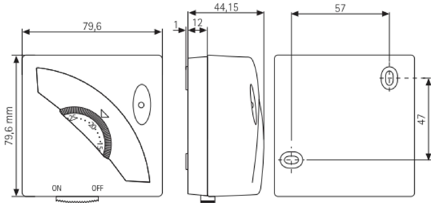
CAMPO DI REGOLAZIONE TEMPERATURA =  $5^{\circ}\div 30^{\circ}\text{C}$
